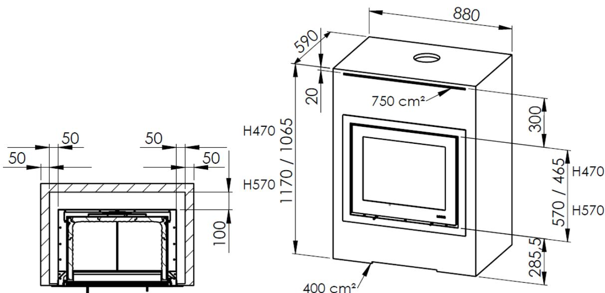
**Insulating material:** Useable are all AGI Q 132 registered insulating material. All measurements are intended as minimum distances.
