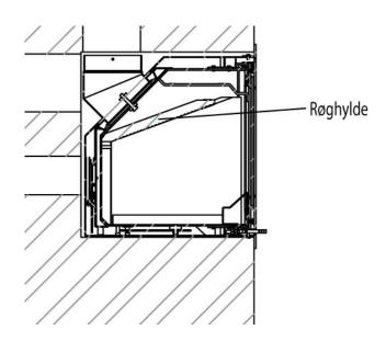
The smoke turn plate is removed by lifting at one side after which it will come clear of the other side and be taken down into the combustion chamber and out through the door. Similarly, it is put in place by moving it up askew at one side and then at the other side, and it is then put in place in the middle.
